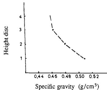
Fig. 2. Axial variation of specific gravity for *Cupressus sempervirens* based on 30 trees.
