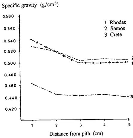
Fig. 3. Patterns of radial variation of specific gravity in the three provenances.
