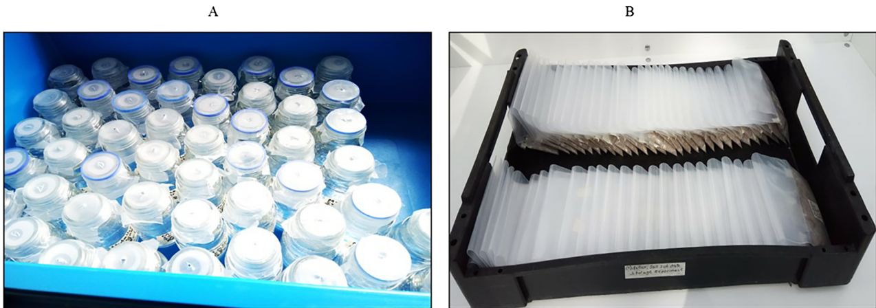
Fig. 1. A: Water substrate in 100 ml bottles; B: Biological bags with 100 g inoculated soil.
